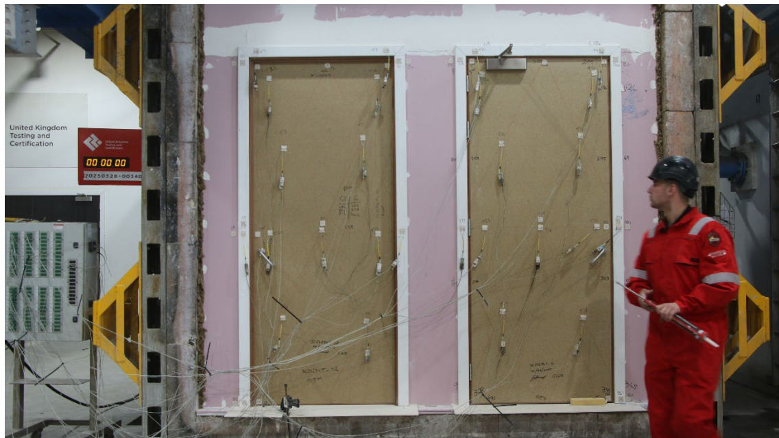
Figure 16 – The unexposed surface of the test construction prior to the commencement of the test
