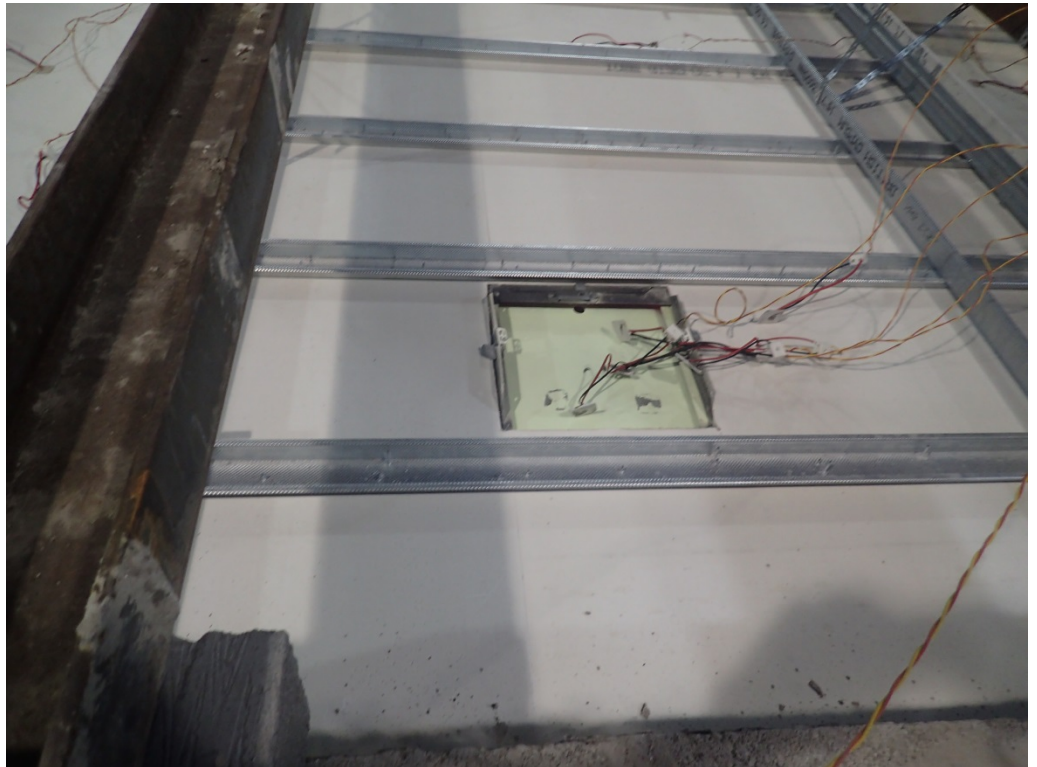
The unexposed face of the assembly during the test
