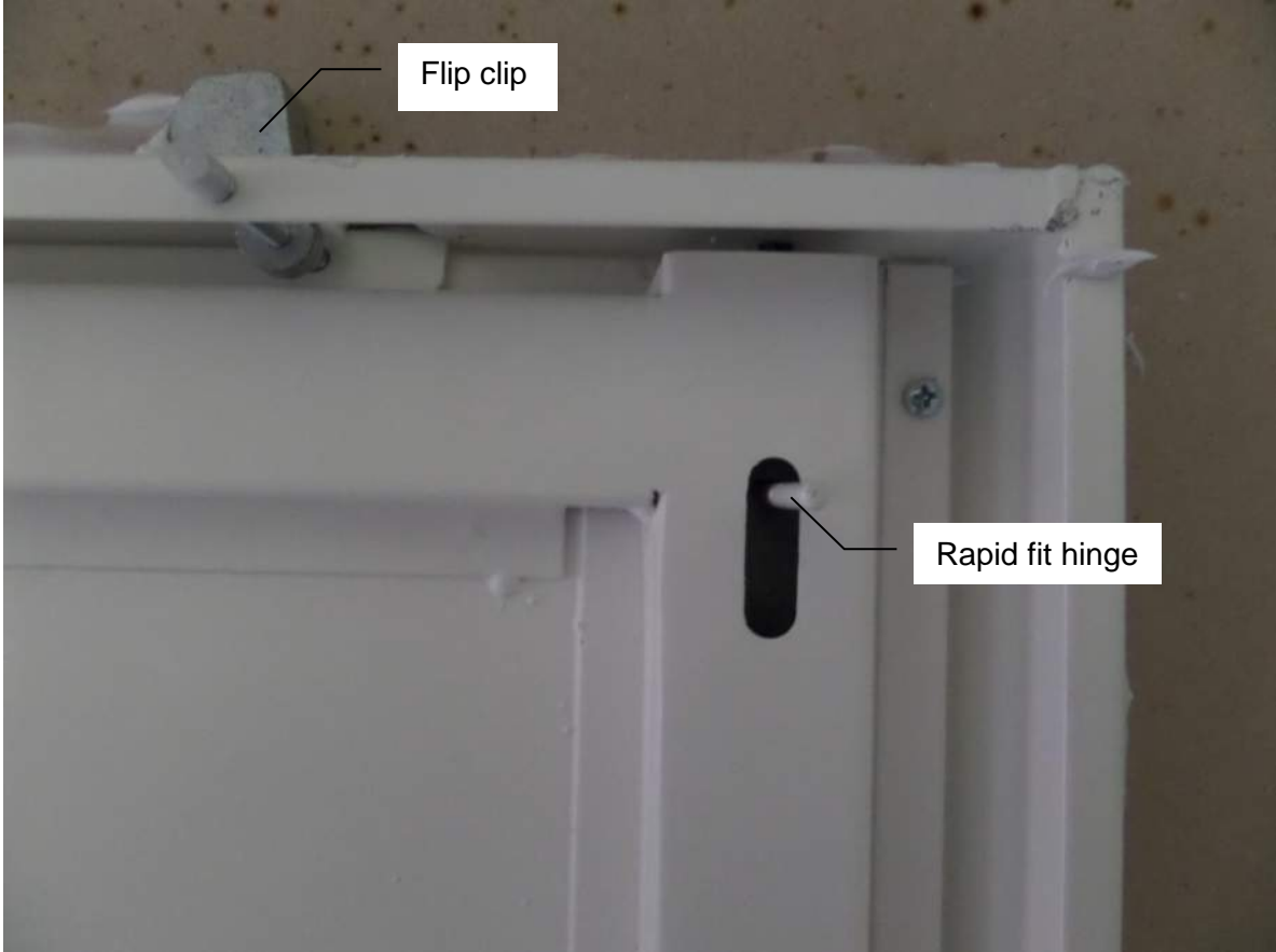
Hardware at top right hand corner of unexposed face.
